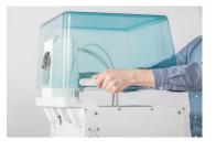
From the front of the printer, place the cover over the filter housing
