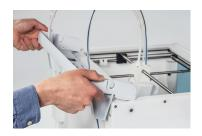
Align the mounting bracket with the back of the Ultimaker S5
