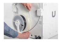
11. Guide the Air Manager cable on the right side around the spool holder and plug it into the **UMB OUT** port at the back of the Ultimaker S5
