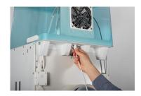
8. Connect the Air Manager cable to the port at the back of the Air Manager
