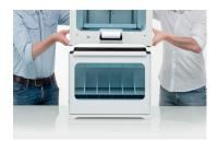
Carefully place the Ultimaker S5 on top of the Material Station
