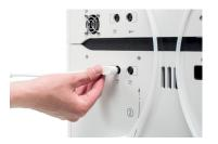
Connect the Material Station cable to the UMB IN port at the back of the Material Station
