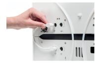
Plug the other end of the cable into the UMB **OUT** port at the back of the Ultimaker S5
