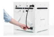
8. Connect the Material Station to the Ultimaker S5 with the power extension cable
