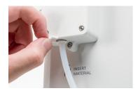
Secure the Bowden tubes with clamp clips 5. Place the spool holder cap into the hole for the spool holder of the Ultimaker S5
