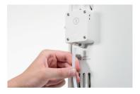
Insert the left Bowden tube into the left feeder, and the right Bowden tube into the right feeder
