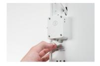
Insert a tube coupling collet in the bottom of each feeder of the Ultimaker S5
