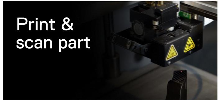
Blacksmith harnesses the power of the X7's existing integrated laser micrometer and a patented intelligent scanning process to securely measure parts as they are printed.
